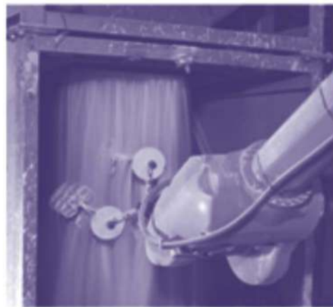
(c) Rain drum used in robotics shelling [ ABB robot]
